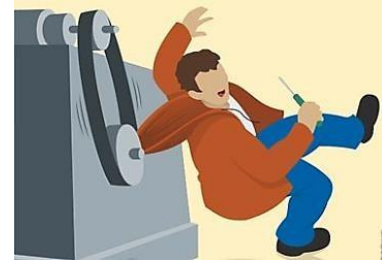
Loose Clothing Entangled Hazard
