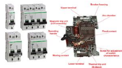
Fig. 4.4 Miniature Circuit Breaker
