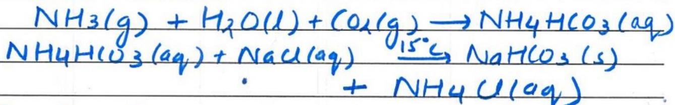
In the lower compartments of the carbonating tower, temperature is lowered to  $15^\circ\text{C}$  due to which  $\text{NaHCO}_3$  precipitates out.  $\text{NH}_4\text{Cl}$  is fed into ammonia recovery tower.
